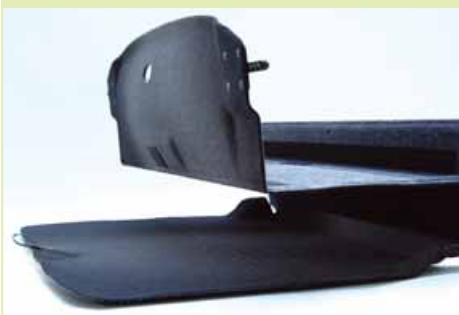
The new luggage compartment cover, into which the convertible top is lowered in fine weather
