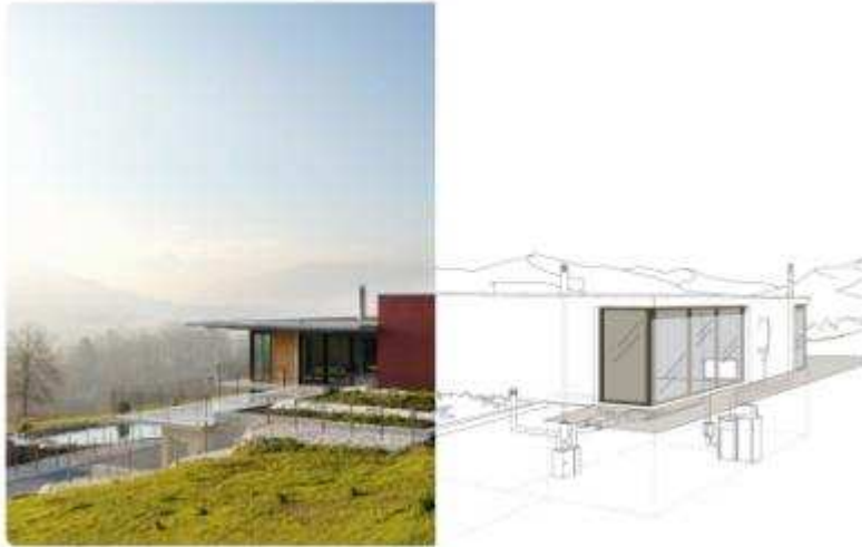
Condensing boiler and heat recovery ventilation
